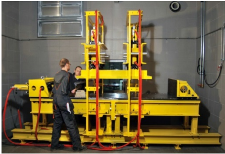
Test bunker with mechanical press with 100 tons max. force and video observation
