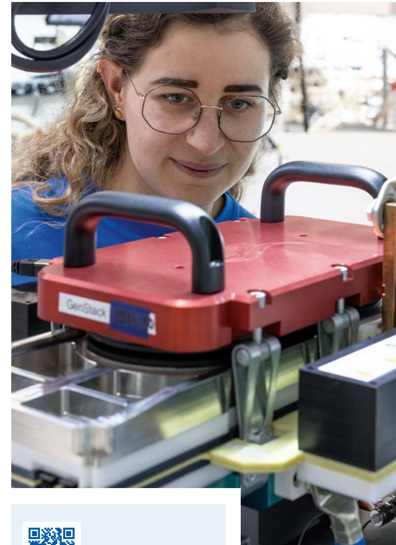
The »generic stack« as a short stack on the test rig and as a full stack with 100 kW output, consisting of 332 individual cells.
