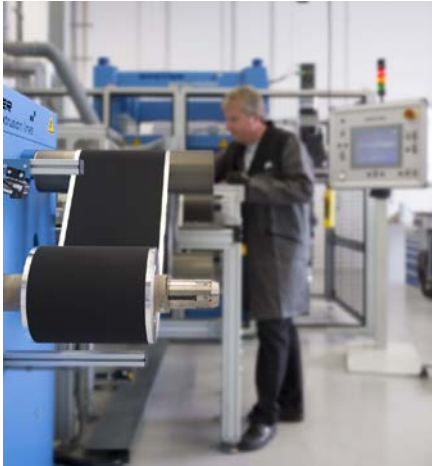
Electrode ready for calendering process. Source: ZSW/Duckek
