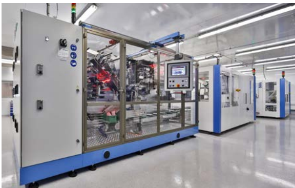
200 m 2 dry room for testing new assembly technologies. Source: ZSW/Duckek
